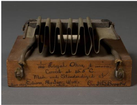
Ten milli-ohm OHM @ 15C. 1887 Edison Machine Works*
